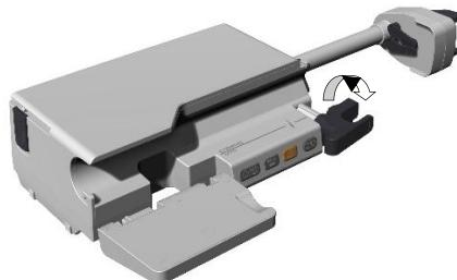
4. Place the air-purged syringe filled with drug solution and connected with the extension tube and scalp vein needle in the syringe pump. The barrel flange of the syringe must be inserted into the barrel flange clamp of the pump. Rotate the syringe clamp counter-clockwise to the original position, and release it so that the clamp presses against the syringe.
