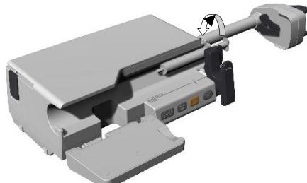
5. Pinching the finger grips, push the push rod to the left to press against the syringe plunger flange. Release the finger grips, the plunger flange of the syringe will be clamped by the plunger flange gripper.
