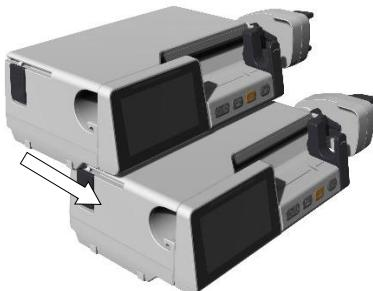
Like the steps shown in **3.1.4 Fit the pole clamp**, multi-channel combined pumps can be fixed on the infusion pole.
