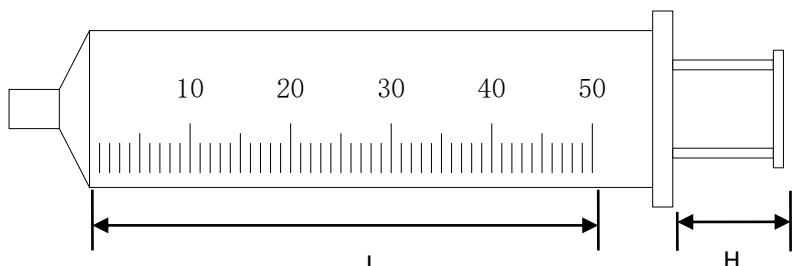
1. As shown in the figure above, push the syringe to 0mL at the end, the length from the 0 mL scale to the nominal scale is I, and H is the length of the plunger.
