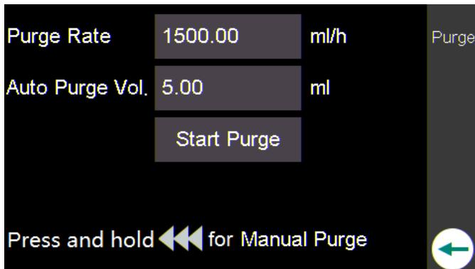
The purge function can be performed only when the device is in the paused or stopped states.
