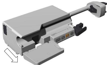
3. Pull the syringe clamp outwards and rotate it clockwise to open the barrel flange clamp.
